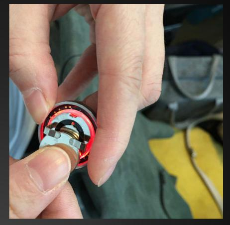
Take the battery out and put it back in again. If the Halo still does not flash red and pink, replace the battery with a new CR1632.
